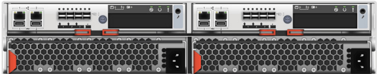
Figure 1-6 IBM Storwize V3700 controller rear view - models 12C and 24C
